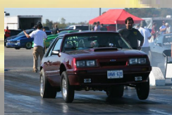
George M 351CI Windsor EFI Victor Jr's Heads PSP Ported Naturally Aspirated Lentech AOD 10.5's @ 127MPH
