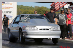
Luis G 400CI SVO Yates C3H Heads Single Turbo Power Glide 8.1's @ 187MPH
