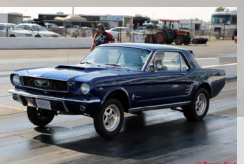
Mike K 327CI Carb Edelbrock Performer RPM Heads Weiand Supercharger C-4 11.3's @ 128MPH
