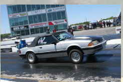
Jeff B 327CI SVO Victor Jr Heads Single Turbo Lentech AOD 9.8's @ 140MPH
